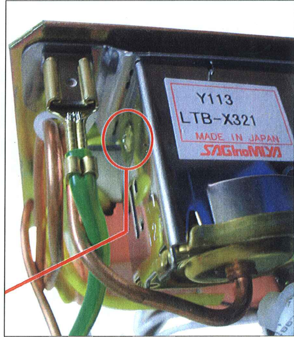
Figure 2: Location of Pressure Switch Adjustment Screw
